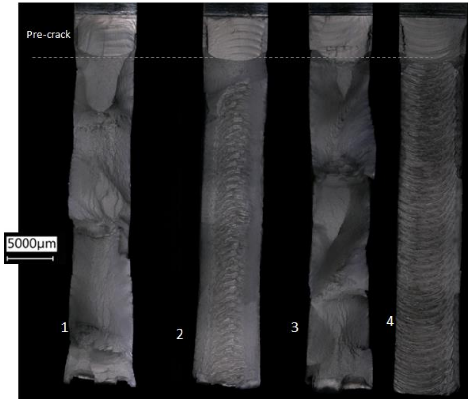
Fig. 3.37 Inner face fracture surfaces of the thinner/faster/T3 FSAM build
