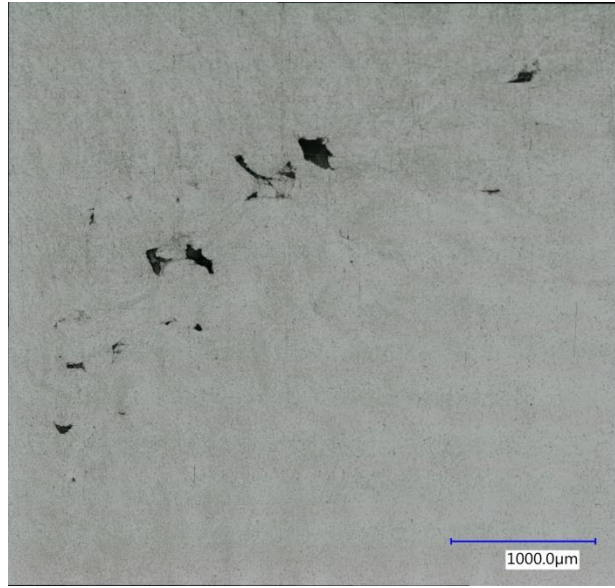
Figure 3.7 Advancing side defects of the slower/thicker/cast build T3 top layer
